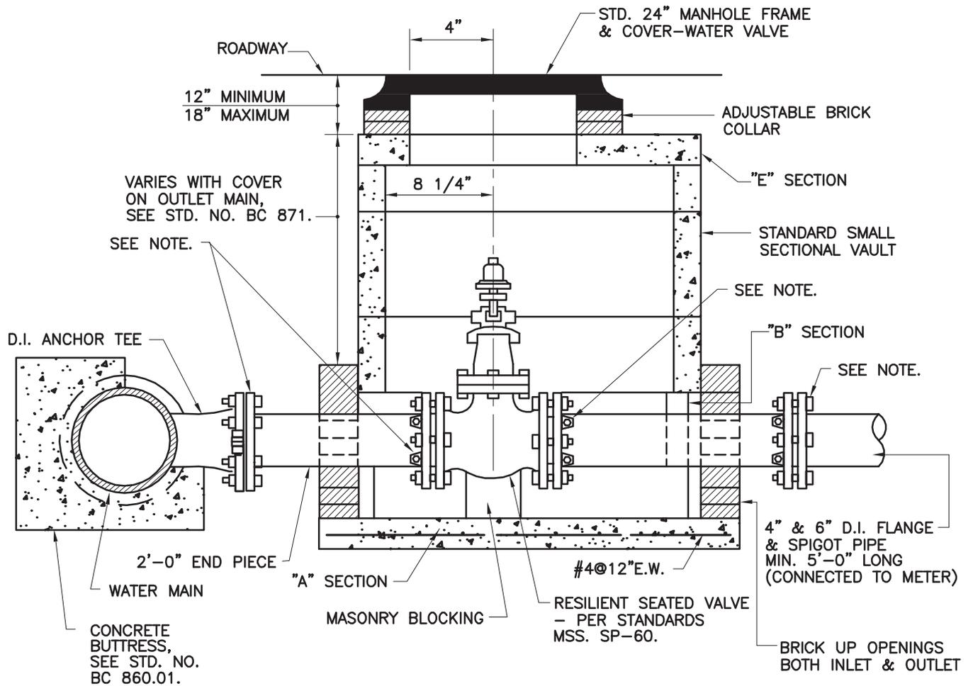
NOTE: ALL JOINTS MUST BE RESTRAINED BACK TO MAIN (ALL-THREAD RODS ARE NOT ACCEPTABLE).
