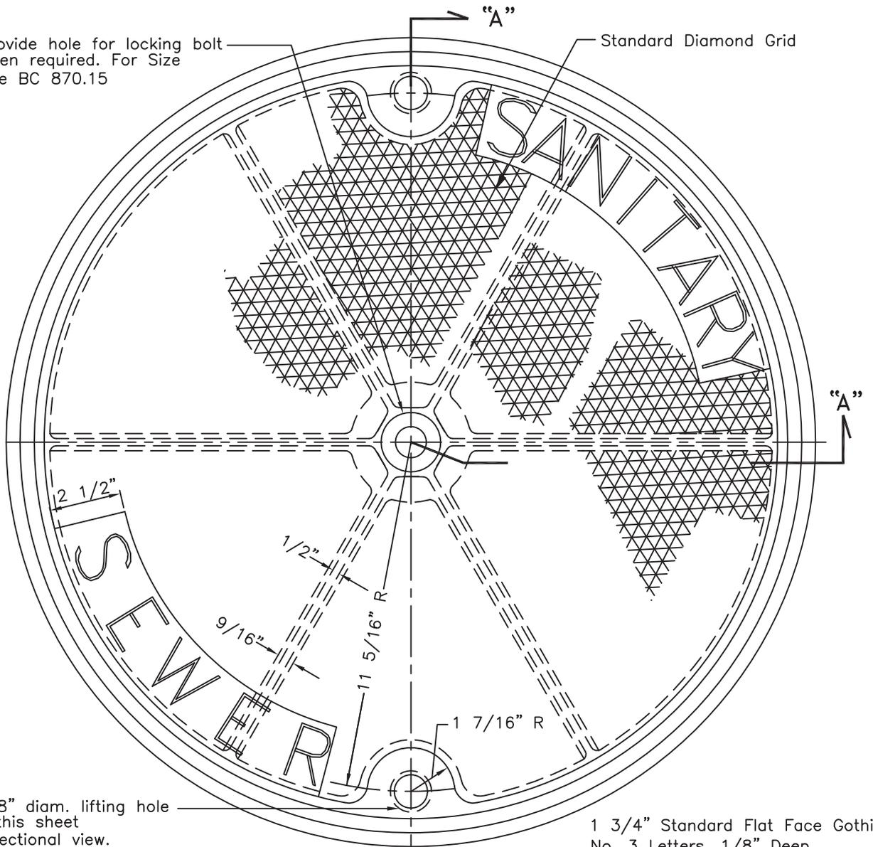
1 1/8" diam. lifting hole See this sheet for sectional view.
