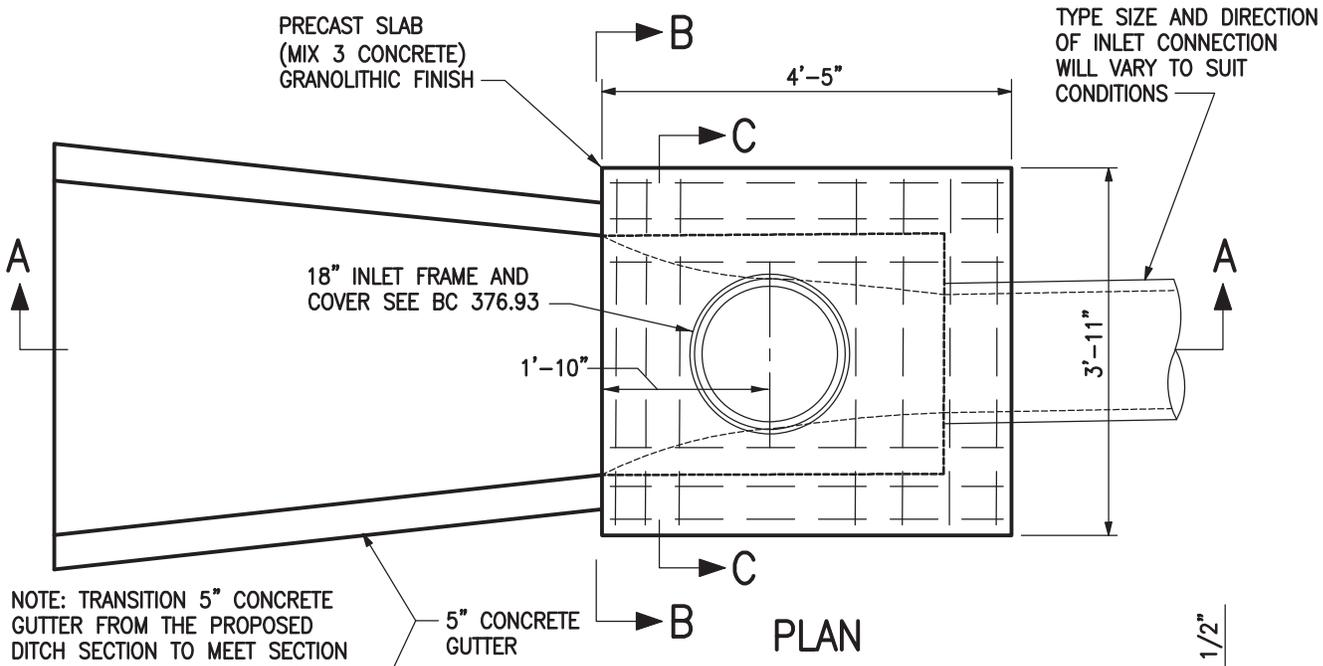
NOTE: TRANSITION 5" CONCRETE GUTTER FROM THE PROPOSED DITCH SECTION TO MEET SECTION B-B AT THE INLET IN SIX(6) FEET.
