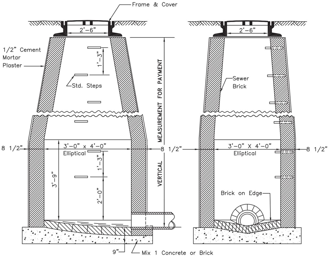
MANHOLE WALL THICKNESS
