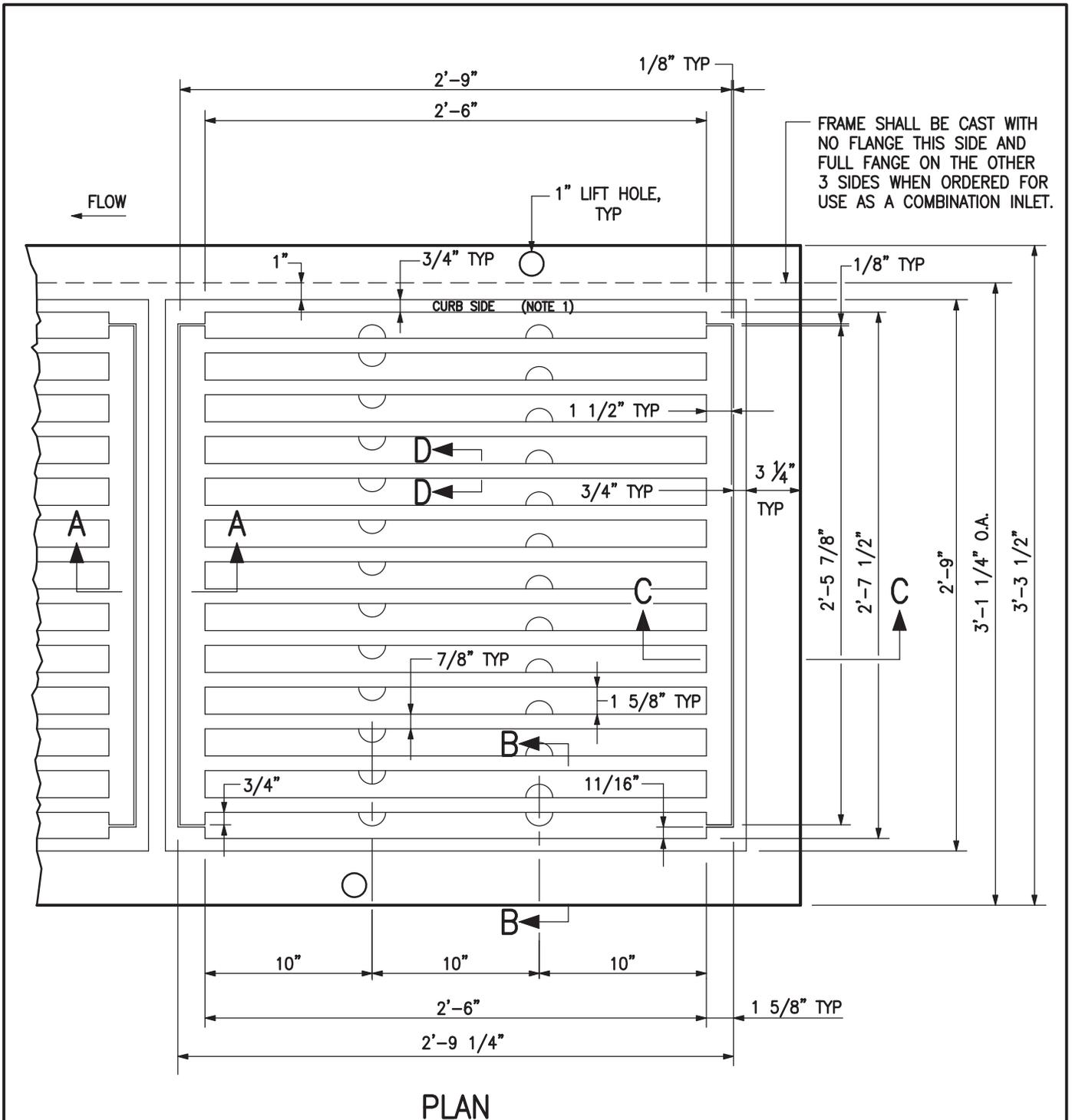
FRAME SHALL BE CAST WITH NO FLANGE THIS SIDE AND FULL FANGE ON THE OTHER 3 SIDES WHEN ORDERED FOR USE AS A COMBINATION INLET.
