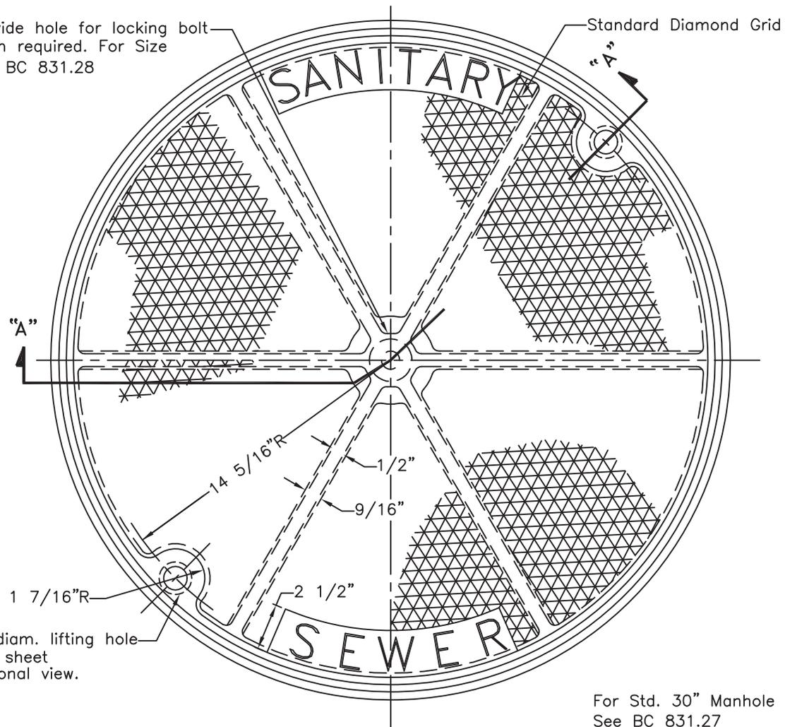
1 1/8" diam. lifting hole See this sheet for sectional view.
