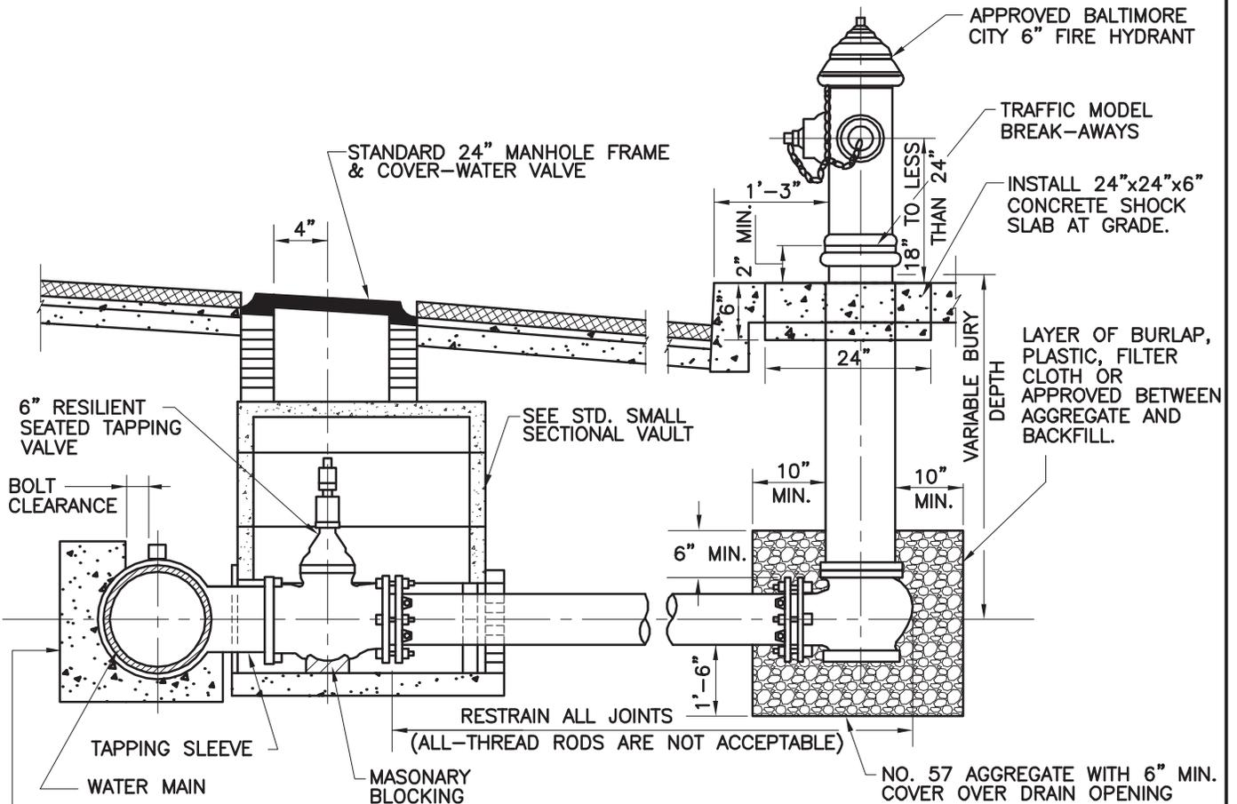
NOTES: 1. BALTIMORE STANDARD FIRE HYDRANT HAS VARIABLE BURY DEPTH. ANY VERTICAL ADJUSTMENT SHALL BE MADE USING BALTIMORE STD. FIRE HYDRANT EXTENSION PIECES.
